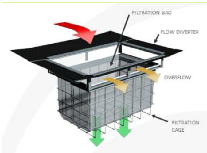
Figure 4 Filter basket operation (Ocean Protect, 2019)
